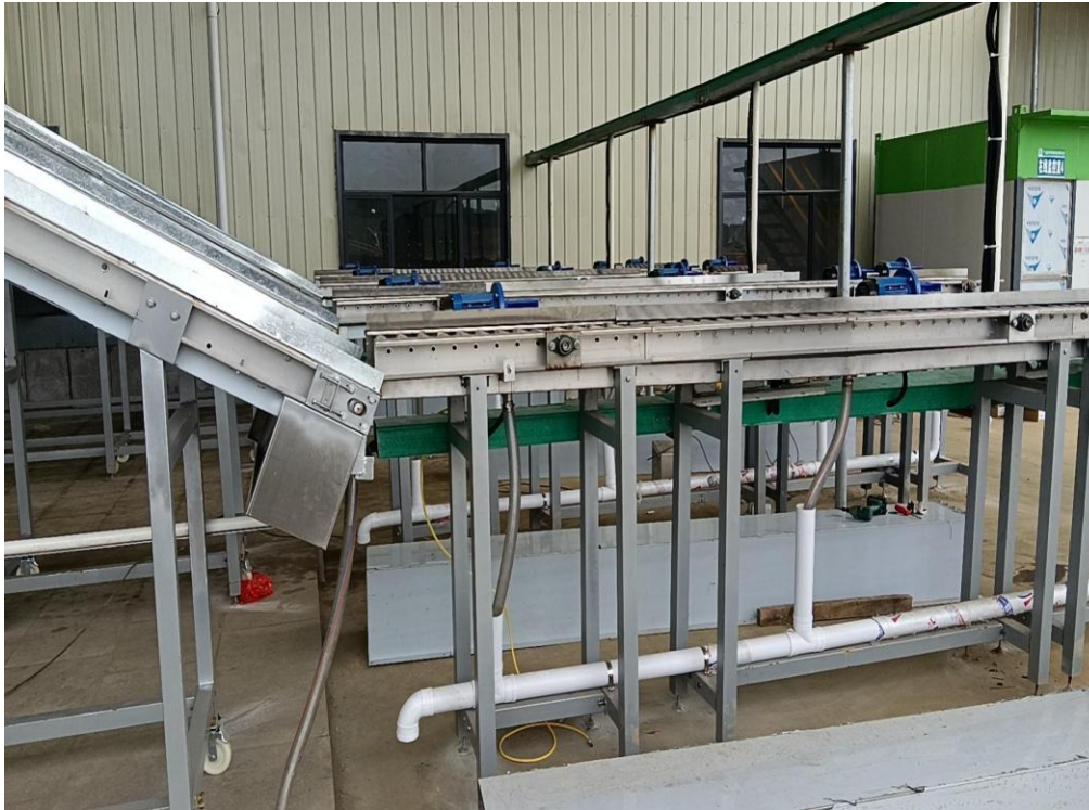
Automatic electrolyte discharging maching for used lead acid batteries
