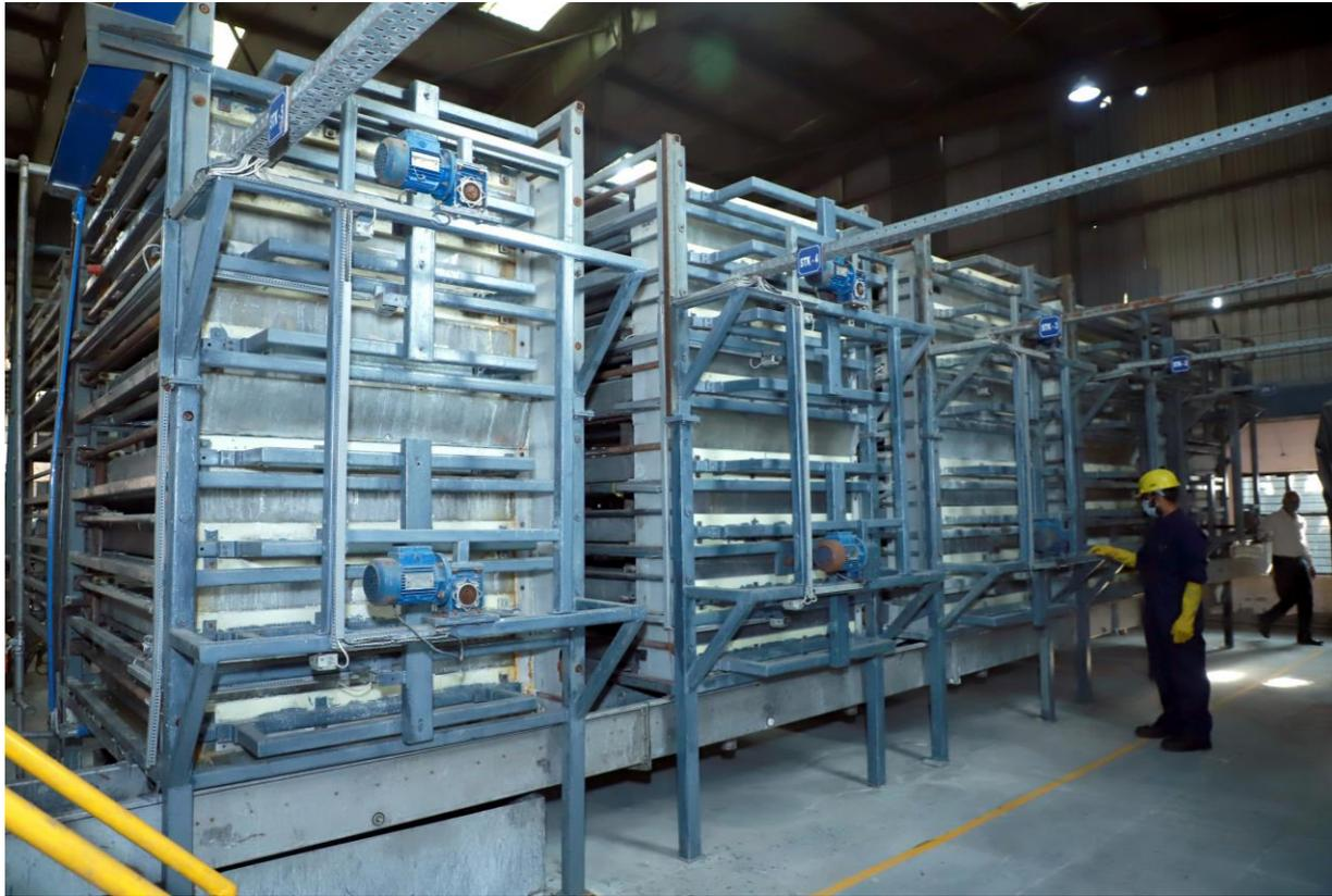
**Lead extracted automatically and safely from modules with minimal operator involvement**
