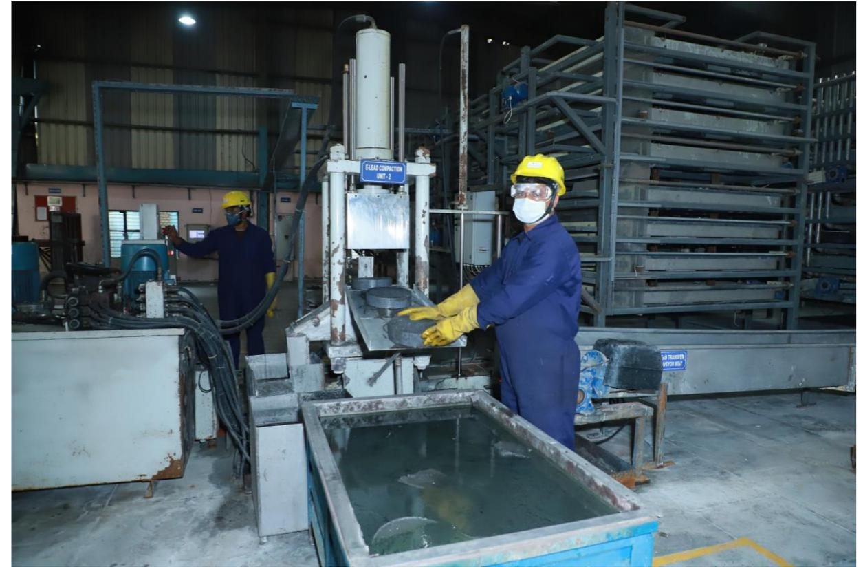
**Operators compacting 'e-lead' bricks for further refinement**
