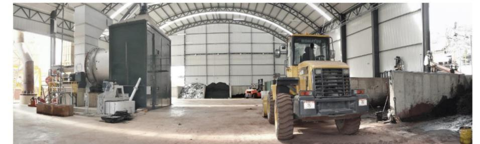
Pb Metals 2012: L to R – refining crucible – rotary furnace – storage bays
